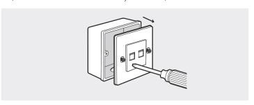
2. Detach the faceplate of the EAP with a screwdriver.
